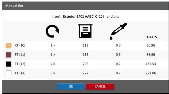
The colorant "TT" is now showing a different way of setting up the pumps to have a more equal way of dosing. It is not anymore giving 1 full stroke + the remaining, but 2x a partial stroke to cover the complete amount without adjusting the scale for the large and small pump.
