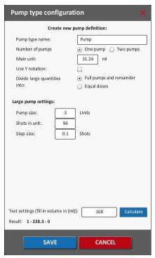
Result: 1 = 1 x full stroke (31.24 x 3) 228.3 = 228 x (31.24 / 96) + 3 x (31.24 / (96 / 0.1)) 0 = n/a, as this is only for a second pump
