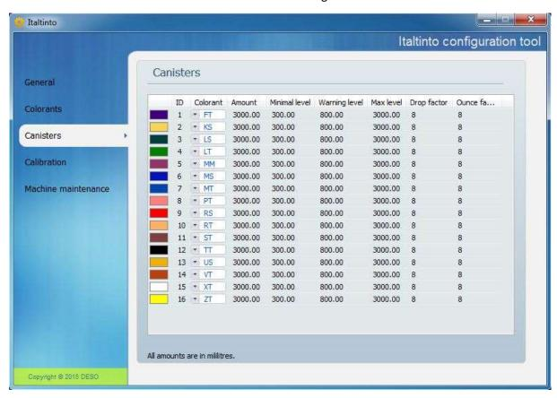
Then comes the calibration. This works in a way that you dispense 3 times a DROP and 3 times an OUNCE. Fill in the weights (you will need a scale for this) and finally click on "Calculate". When everything is fine it will state "Calibration OK". When one or more values are too far off it will give an error message and you must repeat the process.
