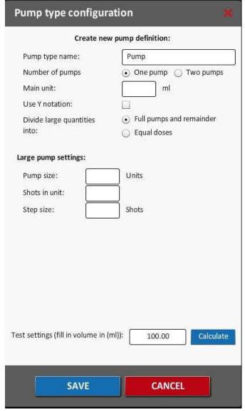
There are several ways to configure the pumps. First it is needed to give the pump a name. This can be anything.
