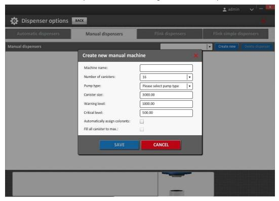
Give the dispenser a name, this can be anything. Select the number of canisters the manual machine has. Now a pump type must be created. This is to configure what kind of pump(s) are available. Select "Please select pump type" and click on "Add new". A new window will appear where the pump type can
