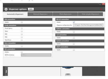
When these settings have been made close Innovatint and start it again. Now it should connect automatically. When it does not check the communication type used for the machine and change it.
