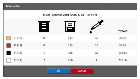
So, in case of colorant "RT" which is at position 10 in the manual machine it needs  $113 \times (31.24 / 96)$  from the large pump and .6 (31.24 / (96 / 0.1)) = 36.96 ml from the small pump.
