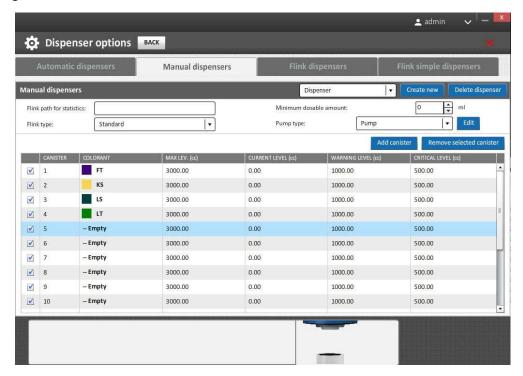
Now the manual machine is configured and can be used. Every time the "Save and dispense" button is clicked a window will come up stating the amounts that should be tinted through the manual machine.
