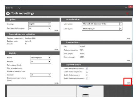
This will open the configuration section for the tinting machines. As you will see only the tab automatic dispensers is available as this is the only connection type that was selected.
