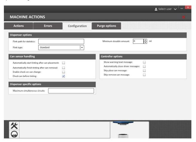
Maximum simultaneous circuits can be set if needed, test values 4, 2 and 1.
