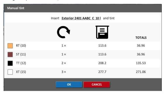
The colorant "TT" is now showing a different way of setting up the pump to have a more equal way of dosing. It is not anymore giving 1 full stroke + the remaining, but 2x a partial stroke to cover the complete amount without adjusting the scale.
