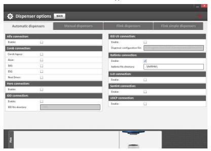
When these settings have been made close Innovatint and start it again. Now it should connect automatically. When it does not check the communication type used for the machine and change it. After that try again to start Innovatint.
